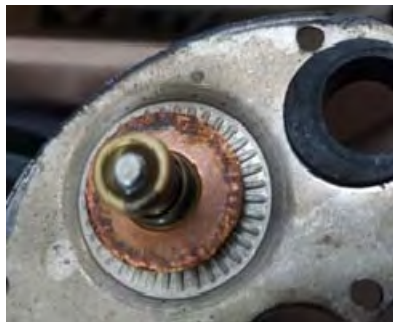
Copper contact disc on MGTC starter - Notice the “chewed-up” area around the Edge of the copper disc!
