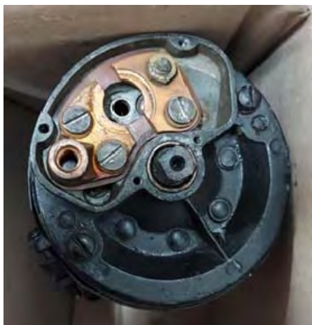
MGTC Starter showing two copper contacts.
