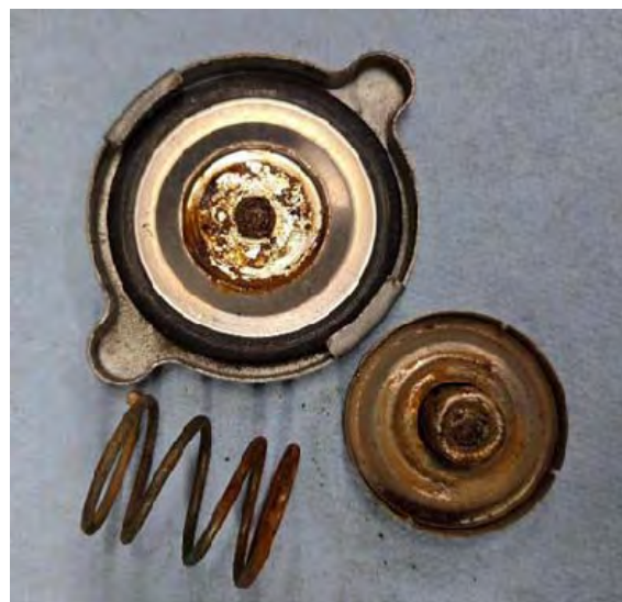
The parts of the radiator cap; the top cover, the spring, and the base which seals to the radiator.
