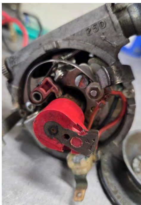
Clean off the rotor contact (left) and file the pitted points (right).
