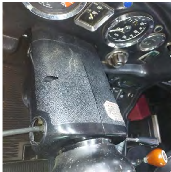
Removing the plastic cowl over the column.
