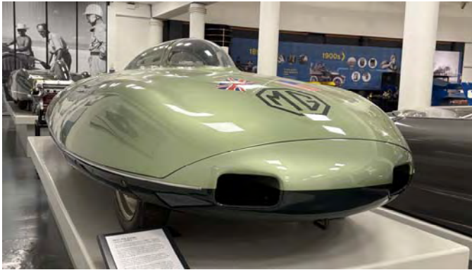
The Land Speed Record 1957 MG EX181 with a 4 cylinder 1506 cc, 300 hp (yes 300!) twin cam MGA engine, which travelled at 255 mph.
