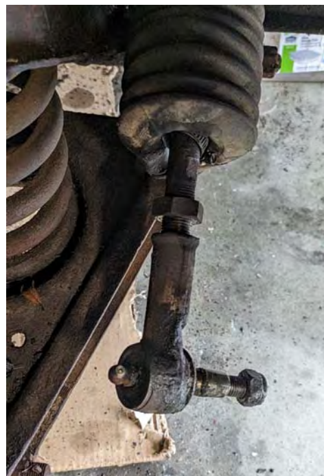
Doug Kennedy's stuck tie rod
