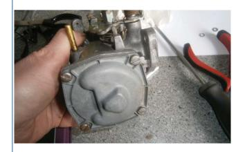
Remove the entire two carb assembly as one unit and lay it on a clean work surface. Be aware that some fuel remains in the carbs so it may leak out as you move the carb assembly around.
