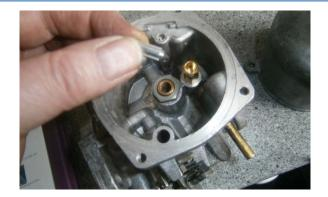
The needle itself can be grasped with fingertips and simply pulled from its seat, which is the brass hex shaped piece screwed into the carburetor.
