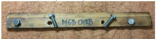
It's pretty simple to make using a scrap of wood long enough to stretch across the fronts of the carb assembly. Mark and drill holes that line up with the bolt holes for the air cleaners, then get four suitable short length bolts from your parts department to complete your new tool. As you can tell, mine has had plenty of use.
