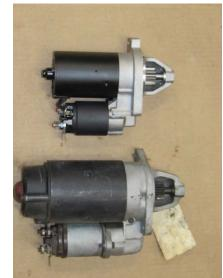
starters were new without the requirement for a core charge or return. The part numbers are: 16164N and Moss 131-220 and it will fit the 1968 and newer MGB.
